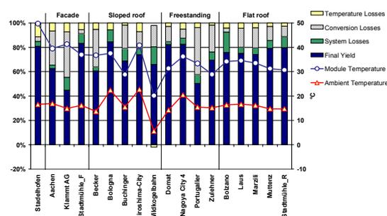
**Figure 3:** Annual yields and losses in percent as well as mean daytime ambient temperature and mean module temperature for 18 grid-connected PV systems with different types of PV array mounting
