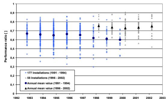
**Figure 5:** Trends of annual performance ratios of 177 residential PV systems installed between 1991 and 1994 compared to 58 new PV systems installed after 1996 in Germany
