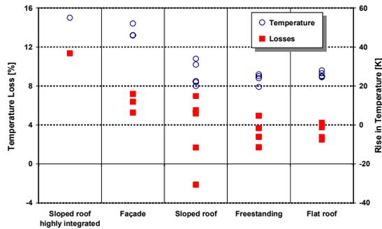
**Figure 4:** Overview of the results for 18 PV systems, showing the temperature losses and the rise in module temperature from ambient temperature (in K at 1000 W/m<sup>2</sup>) grouped by the type of PV array mounting
