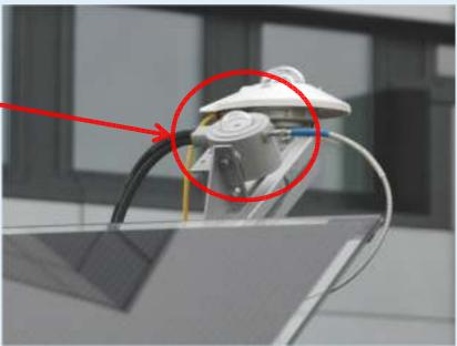
Outdoor spectrometer measurements: 300nm – 1600nm In module plane, 35° tilted facing south (direction influences result)
