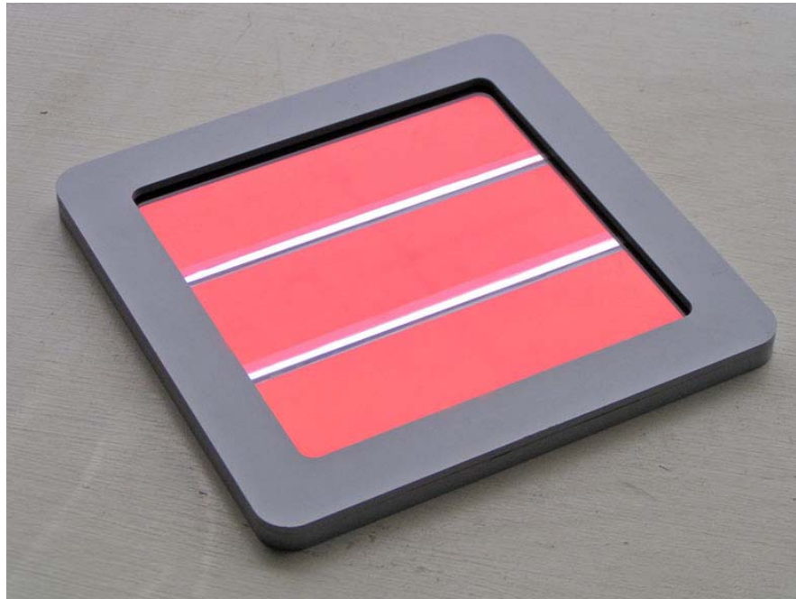
Figure 11: Organic solar cell developed at CSIRO. This technology is compatible with a low cost, high speed printing process that could significantly reduce the cost to the consumer.
