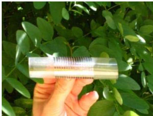
Figure 8: Prototype of ANU lightweight flexible solar module based on ultrathin crystalline Si solar cells.
