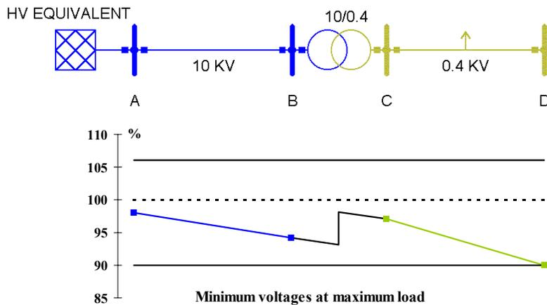
Figure 6 Minimum voltages at maximum load in the simplified power system
