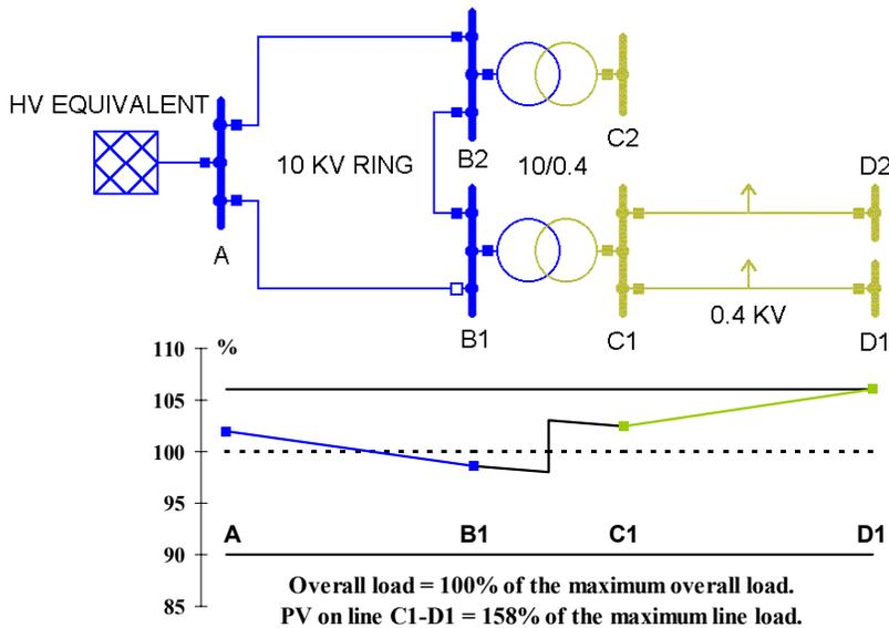
Figure 11 An amount of PV penetration equal to 158% of the load is acceptable at maximum load
