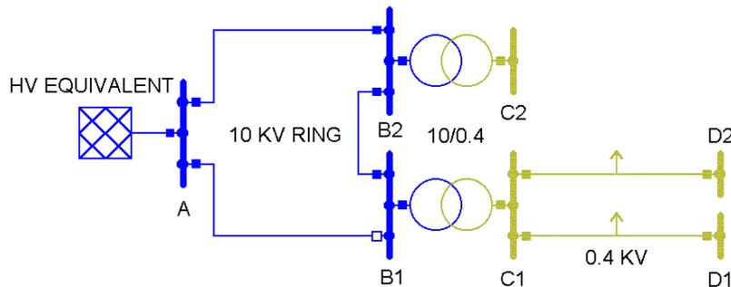
Figure 8 Typical configuration of the MV/LV power system
