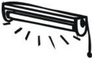
• Undervoltage will cause a fluorescent lamp to oscillate continuously preventing start up. In addition, using glow starters, the consumption can continuously be about 5 times the nominal. This abnormal mode can sometimes damage the starter !
