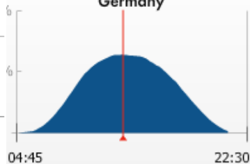
Daily Variation of PV Power in % of the Total Installed PV Power in Germany
