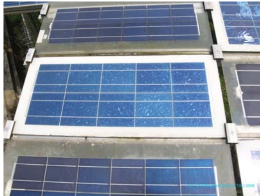
Degradation of the encapsulant after 12 months at the tropical test site
