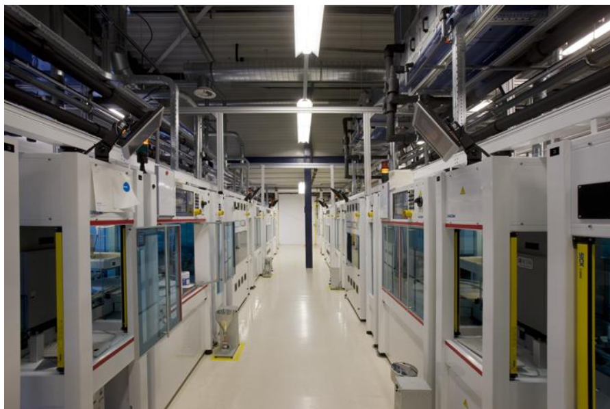
Figure 3-1: Production line of crystalline PV modules by Solland Solar
