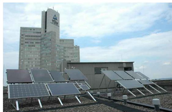
**Figure 1:** Photo of the outdoor test field for energy yield measurements of ten thin-film and two crystalline PV modules
