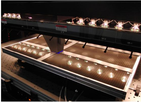
**Figure 7:** Non-destructive spectral response measurement station at TÜV Rheinland, Cologne
